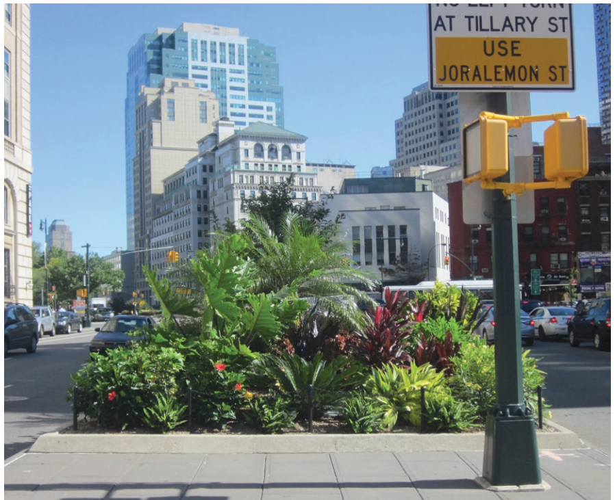
Planted median. Low plantings are located near the intersection to allow better visibility. Contrasting colors and texture add interest: Adams Street, Brooklyn (Credit: DPR)
